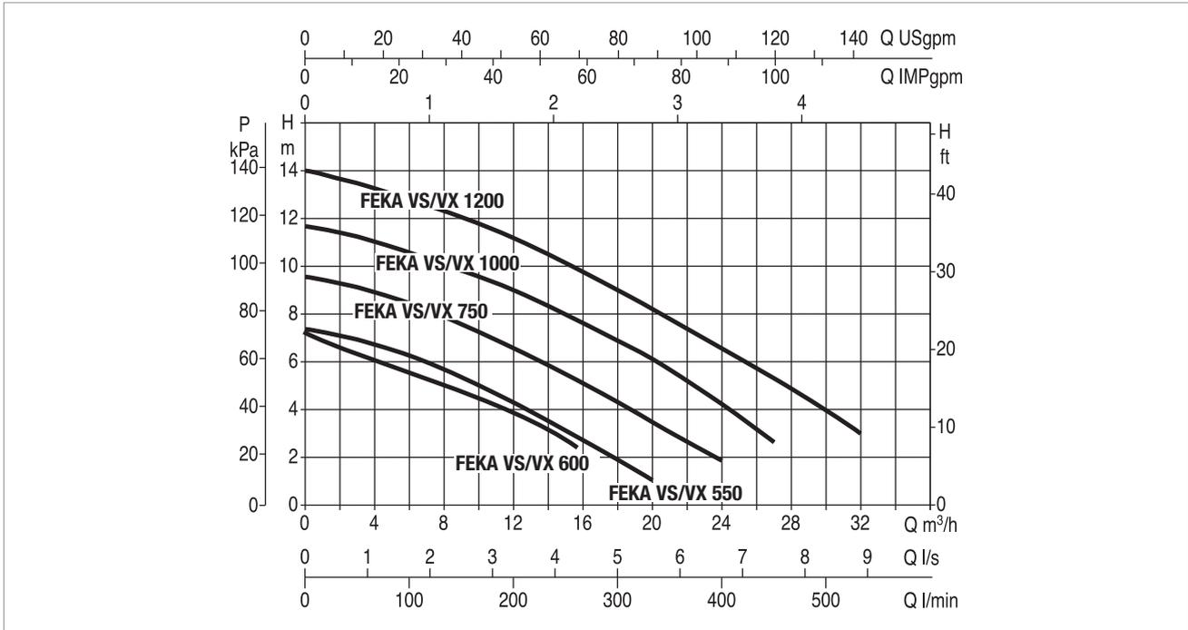
Performance curves are based on kinematic viscosity values = 1 mm²/s and density of 1000 Kg/m³. Curve tolerance in accordance with ISO 9906.
