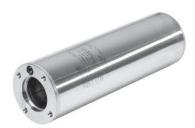
Stator housed in an outer casing in AISI 304L. The stator has 24 slots to ensure better elasticity and smooth operation; the copper conductors have a double layer of Class H insulating enamel. Thermal protection is included in the motor of 0,5 HP to 1,5 HP in the 50 Hz version of 0,5 HP.
